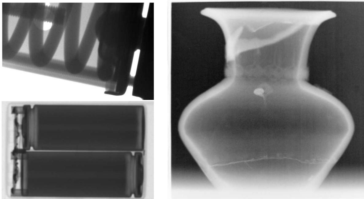
Fig. 2. (a) 300 kV pulsed x-ray images (Colorado Mines 2014); (b) 200x200mm neutron image on 1.3 MW TRIGA reactor (TINT 2014)
