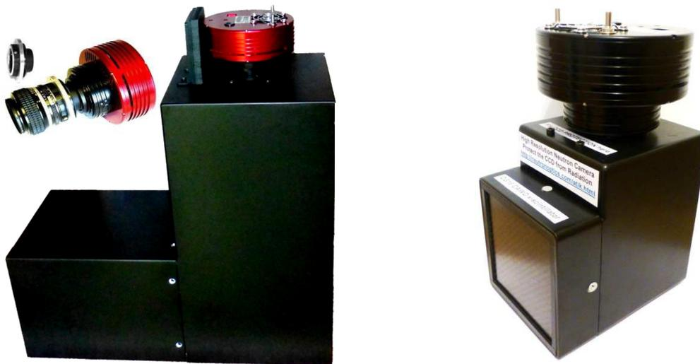
Fig. 1. (a) 200x200mm high resolution neutron or x-ray camera;
