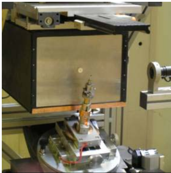
Fig. 2 OrientExpress at ILL is a CCD detector on a continuous white neutron beam from a thermal guide (Ouladdiaf et al 16 ).
