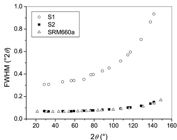
**Figure 1** FWHM versus diffraction angle, as obtained from laboratory X-ray measurements, for three samples:  $\text{CeO}_2$  with broadened lines (sample S1), annealed  $\text{CeO}_2$  used to correct for instrumental effects (sample S2), and new NIST SRM660a  $\text{LaB}_6$ .
