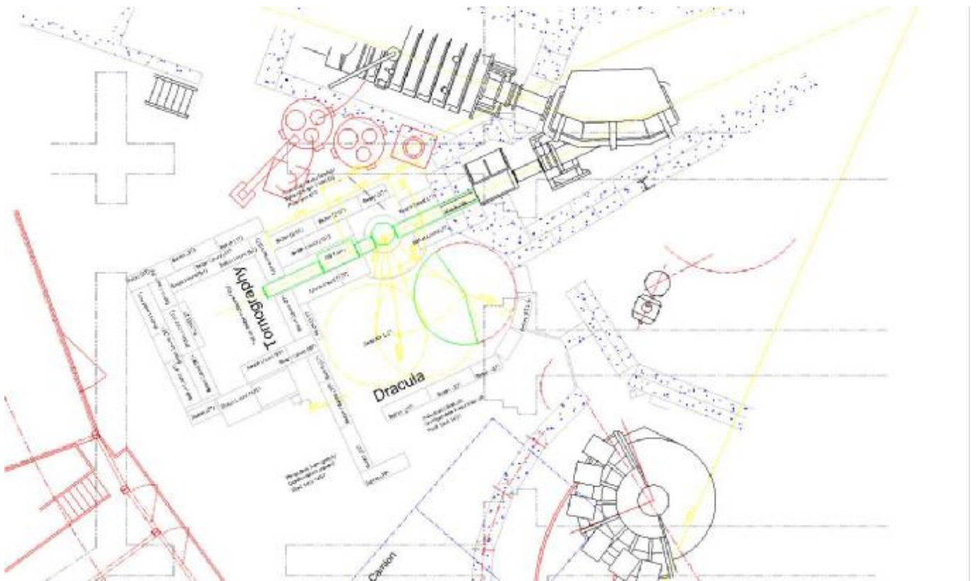
Fig. 1b Option B: Dracula would displace the tomography station on the 200mm diameter high flux H9 Lohengrin beam tube.
