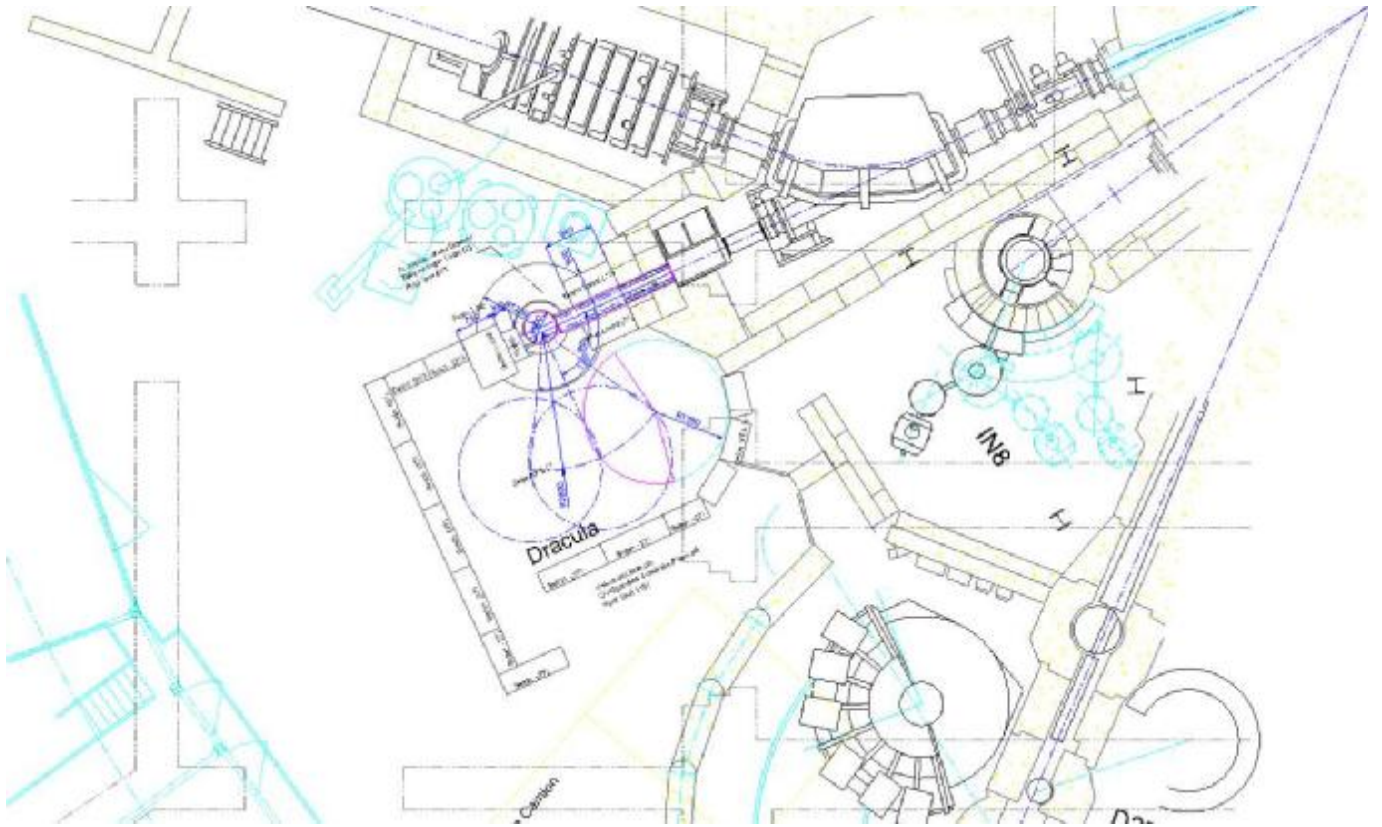
Fig. 1a Option A: Dracula would replace the tomography station on the 200mm diameter high flux H9 Lohengrin beam tube.
