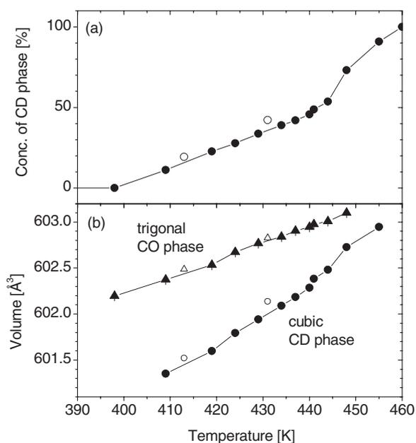
**Figure 2.** Temperature dependence of the CD phase concentration (a), the unit-cell volume of the trigonal CO phase (triangles) (b) and the unit-cell volume (multiplied by 1.5) of the cubic CD phase (circles) (b). All these values are determined from Rietveld analysis of powder neutron diffraction data of  $\text{CaMn}_7\text{O}_{12}$ . The full symbols show values measured with warming between the temperature steps, the open symbols those measured with cooling.
