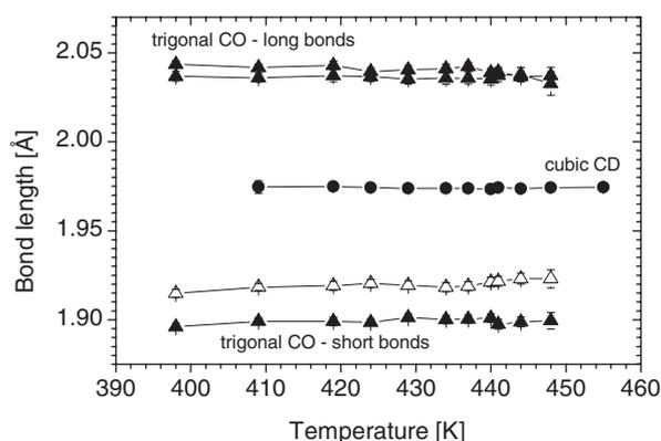
**Figure 4.** Length of the Mn–O bonds for Mn ions located in the B sublattice of  $\text{CaMn}_7\text{O}_{12}$ . The Jahn–Teller-distorted  $\text{Mn}^{3+}$  in (9d) trigonal (CO) sites have three different Mn–O bondlengths (solid triangles) and the undistorted  $\text{Mn}^{4+}$  in (3b) trigonal (CO) sites have one Mn–O bondlength (open triangles). The corresponding Mn ions in the CD cubic phase located in (8c) sites have one bondlength (circles).
