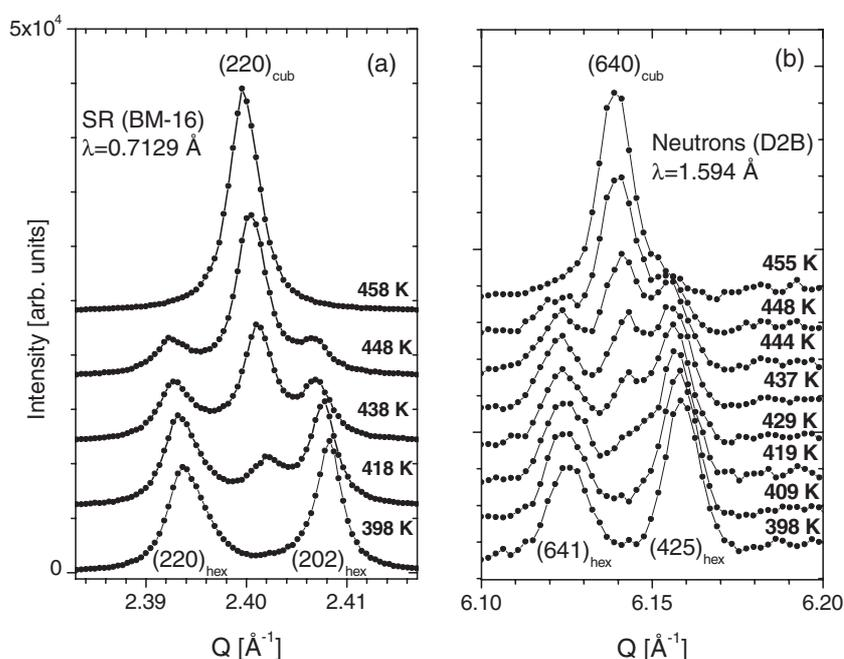
**Figure 1.** Representative parts of the SR (a) and neutron (b) powder diffraction patterns of  $\text{CaMn}_7\text{O}_{12}$  measured in the PS region. Solid circles represent measured data and the curves are shown to guide the eye.  $Q$  is the length of the scattering vector calculated as  $Q = (4\pi/\lambda) \sin \theta$ , where the scattering angle is  $2\theta$ . The patterns measured at different temperatures are vertically shifted for clarity.
