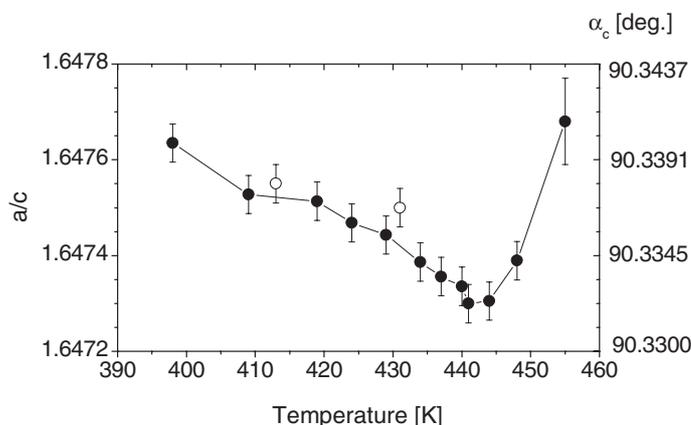
**Figure 3.** Temperature dependence of the  $a/c$  lattice parameter ratio in the CO trigonal phase of  $\text{CaMn}_7\text{O}_{12}$  determined from neutron powder diffraction data. The right-hand scale shows the corresponding values of the angle between the pseudo-cubic axes (see text). The full symbols show values measured on warming while the open symbols those on cooling.
