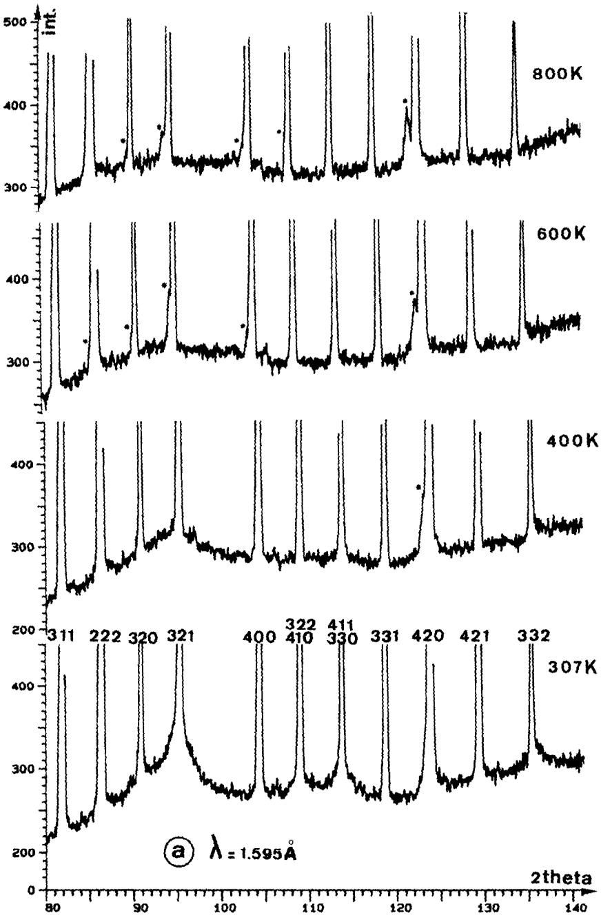
FIG. 4. Evolution of some neutron diffraction lines between 800 and 5 K. (a) Diffraction patterns recorded on D2B. (b) Diffraction patterns recorded on D1A. \* Parasite lines due to an oxygen-deficient phase of PMN formed at high temperature.
