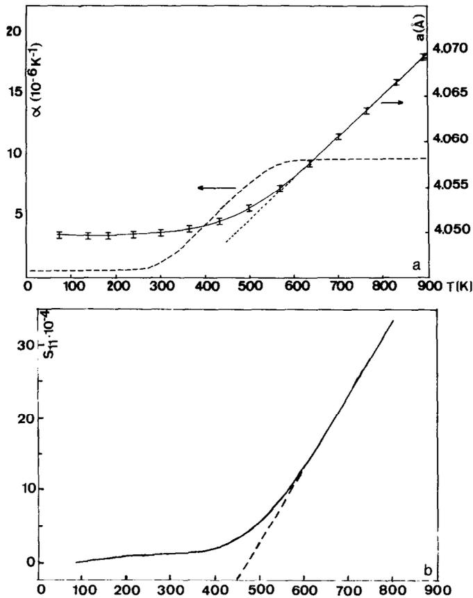
FIG. 5. (a) Evolution of the cubic cell parameter and of thermal expansion  $\alpha = 1/L \cdot (\Delta L/\Delta T)$  vs temperature. (b) Thermal strain  $S_{11} = \Delta L/L$  vs temperature for PMN according to (10).
