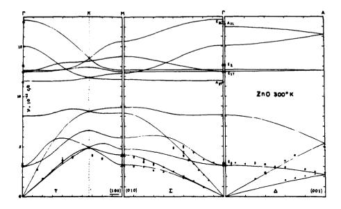
FIG. 1. Phonon dispersion in ZnO at 298°K predicted by a shell model based on elastic constants and Raman spectrum, with measured frequencies.
