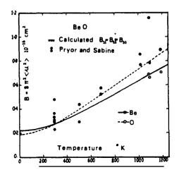
FIG. 2. BeO B-factors for a shell model with measurements of Pryor and Sabine. 14
