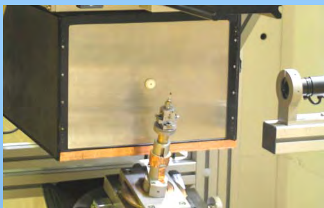
OrientExpress, prototype cooled CCD neutron detector at ILL
